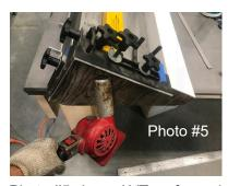
Photo #5 shows LVT preformed treads on a cutting block being heated from below so cutting becomes quicker, using less effort.
